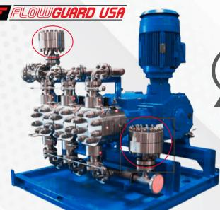
FlowGuard pulsation dampeners use a small volume of gas, typically nitrogen, contained within a flexible membrane inside a non-corrosive shell. When a pulse from the pump occurs, the gas is slightly compressed. As the flow decreases, the stored pulse is released back into the line, resulting in a smooth flow and minimizing pressure fluctuations.
